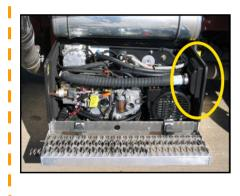
2007 and 2008 Frigette APU's have plastic housings located on the right side of the box. To inspect the air filter elements, remove the lid and pull the vinyl trim lock strip off the right side edge of the box.
